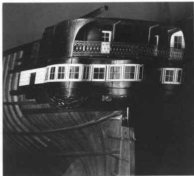
37. ( La Chartre ). This frigate was a 30-pdr vessel of the 3 rd Rank, and it provides an early and very ugly example of the round stern. The multiplicity of lights on the main deck, and the effect of three towers formed by the quarter-galleries to port and starboard and the space needed for the rudderhead amidships (the counter no longer exists), combine to give an impression of a "folly"! There is a quarterdeck cabin with access to a stern-gallery and the upper level of the quarter-galleries; the latter are entirely berthed up, providing a strange contrast with the plethora of lights below. In short, the effect is as bizarre as it is ugly, and it may be that it was simply a bungled attempt to copy an English design.
