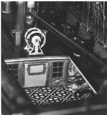
42-43. ( La Flore ). Two views of the great cabin, the domain of the Captain. At the level of the quarterdeck can be seen the doorway leading to the canvas shelter (not shown) over the upper-finishing of the quarter-gallery. There is also an arms chest and a poultry-coop with feeders hard up against the stern. Note that there is no ensign-staff any more, since it is flown from the end of the gaff.
