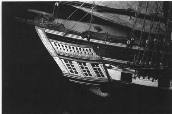
32. ( Unnamed 18-dr frigate, ca 1800 ). View of the quarter-gallery. Note the way it is tucked into the angle formed by the projection of the horseshoe arch and the frigate's side. The quarter-lights are false, and the doorway leads off from the main deck.
