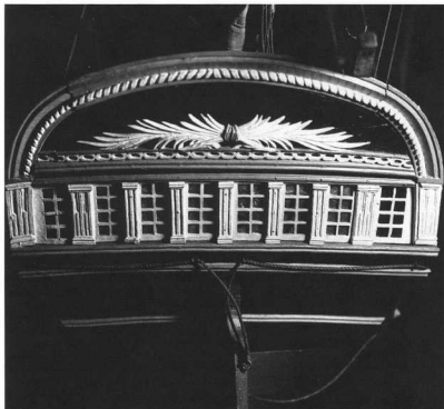
34. ( Unnamed 18-dr frigate, ca 1800 ). The stern. Although not particularly well executed, it nevertheless provides a good example of the typical horseshoe shape combined with pilasters between the sternlights (the outboard lights are false). The taffarel is too small for anything other than a simple motif of two palm leaves linked by a knot; the emblem which originally occupied the space above has been lost.
