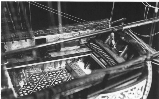
42-43. ( La Flore ). Two views of the great cabin, the domain of the Captain. At the level of the quarterdeck can be seen the doorway leading to the canvas shelter (not shown) over the upper-finishing of the quarter-gallery. There is also an arms chest and a poultry-coop with feeders hard up against the stern. Note that there is no ensign-staff any more, since it is flown from the end of the gaff.
