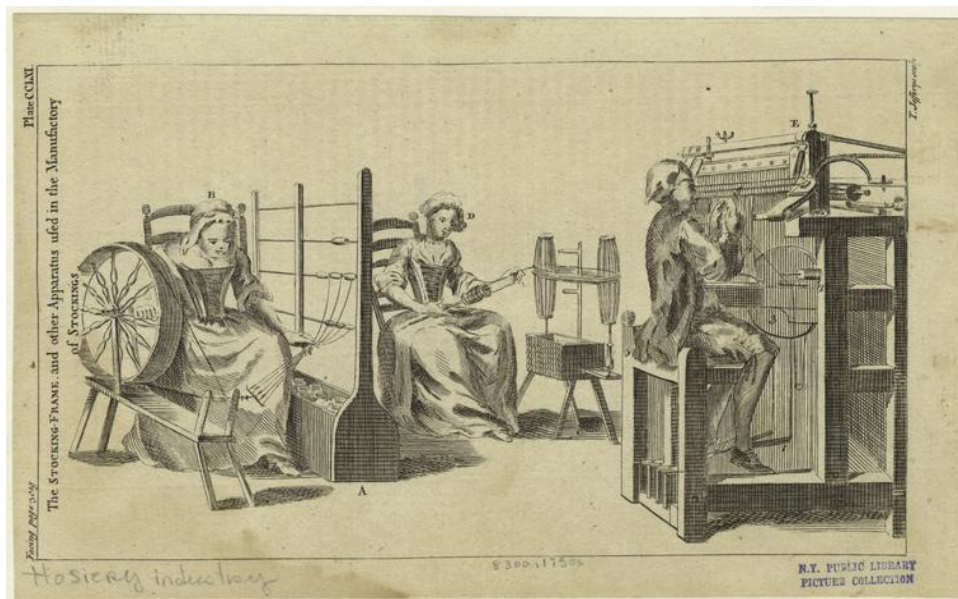
The stocking-frame and other apparatus used in the manufactory of stockings. (1754-1755)
