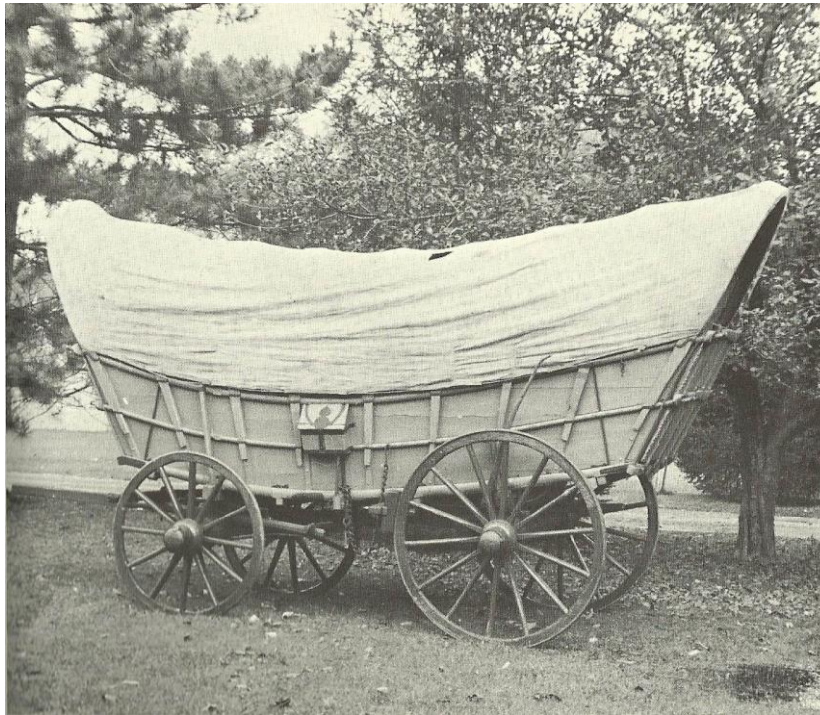
“A relatively small but graceful nine-bow Conestoga owned by [the late] D.H. Berkebile.” George Shumway, Edward Durell, and Howard C. Frey, Conestoga Wagon 1750-1850 (York, Pa., 1964), 51.
