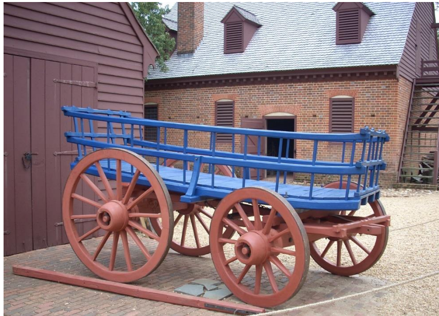
The "large English" wagons used by the British army in 1776 and 1777 were likely similar in size and style to English carrier's wagons of the period. This example, built at Colonial Williamsburg and completed in late 2007, weighs approximately 2,700 pounds. (Wagon constructed by the Colonial Williamsburg wheelwright shop; photo courtesy of same.)
