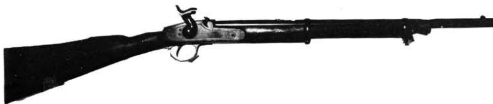
.577 Muzzle-loading Percussion Carbine issued to the Artillery in 1858. It embodied the Enfield 3-grooved barrel
