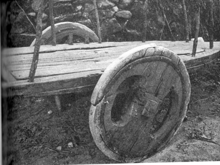
1. A typical ox-cart of the type used by Wellington. The wooden axle was solidly connected to both wheels, and revolved in two wooden journals.
