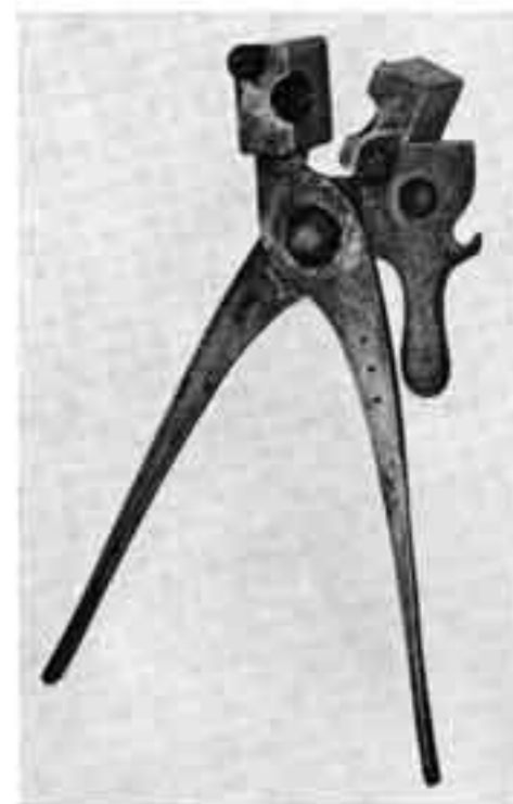
Bullet mould, mid-19th century, for casting lead bullets, calibre 0.577 in., to be used in the percussion Enfield rifle.
